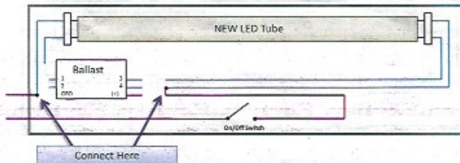
Step 6: Connect Ground wire to either Wire 1 or 2 as shown
